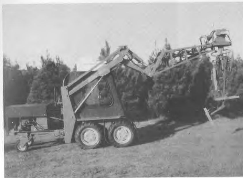
Figure 18: In the South, where topography is gentle and the summers are long and hot, shearing machines have been developed to shape Virginia pine. This species requires at least 2 shearings each summer. Photo credit: Murphy-Matic, Inc.
