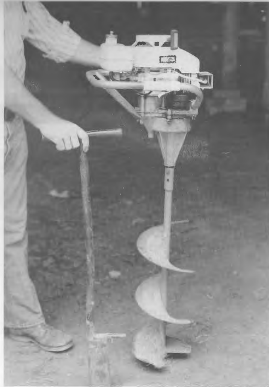
Figure 11: The Old Standard (OST) planting bar has a wedge-shaped blade that tapers to a straight edge at the bottom. The gasoline-powered portable auger is best for planting large transplants or potted trees. Both tools operate best in light-textured soils.
