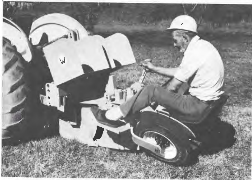
Figure 16: Transplanter for use in contour terrain planting. The packing wheels can be turned up the hillside to keep the tires from running over planted seedlings. Rear packing section is spring loaded to keep the packing wheels on the ground for packing pressure at all times. Photo credit: R. A. Whitfield Mfg.
