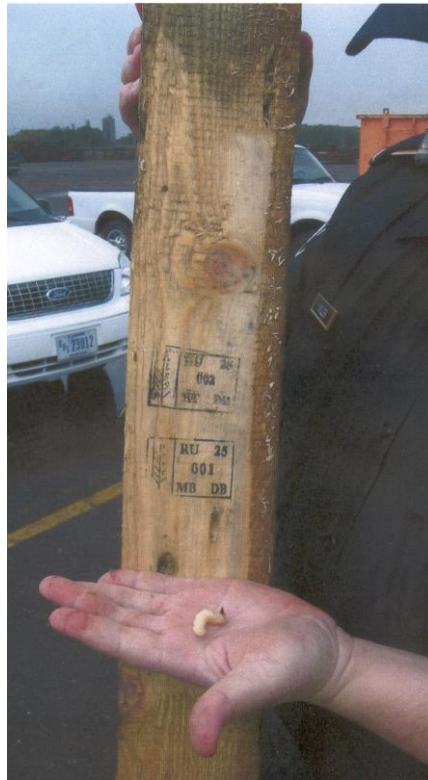
Live larva found in wood packaging with ISPM mark; Photograph courtesy of Oregon Department of Agriculture
