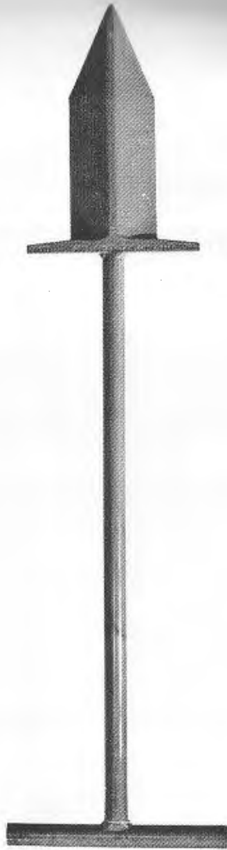
Figure 12: The KBC planting bar features a blade with a wide, triangular cross section that tapers to a point in the last 4 inches. The KBC bar creates a tapered hole that can accommodate large, bare-root seedlings. It is well adapted to hard, rocky soils.
